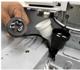
8. Finally, you can connect the end of the IEC C13 cable and extension cord to the battery.
